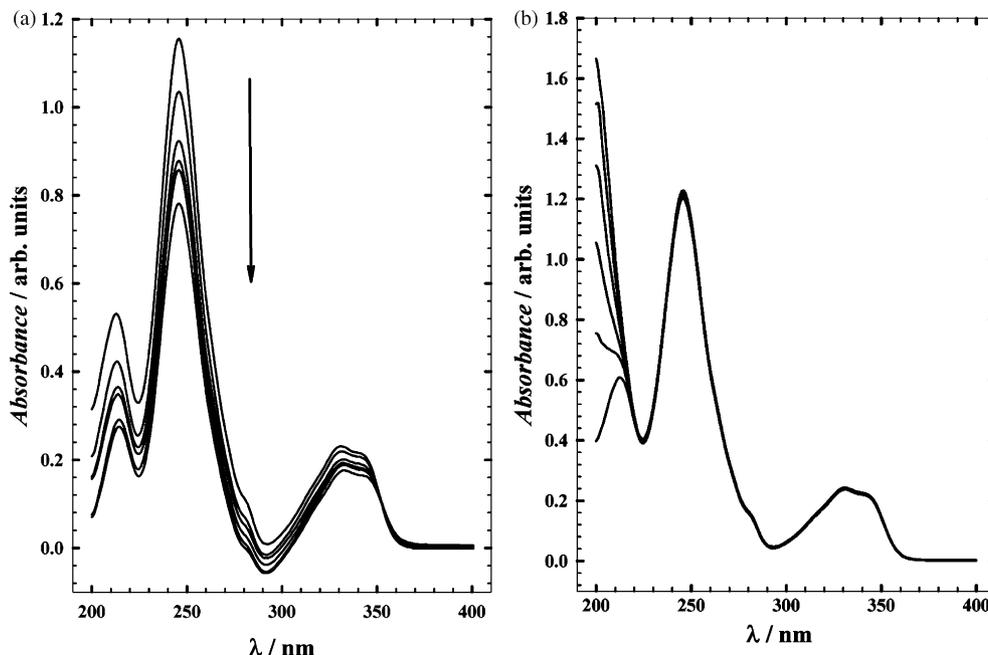
Fig. 4. (a) The effect of different concentrations of SDS surfactant on the absorption spectrum of  $4.76 \times 10^{-5} \text{ mol L}^{-1}$  terazosin dye in aqueous universal buffer, pH 2.0. (b) The effect of different concentrations of CTAB surfactant on the absorption spectrum of  $4.76 \times 10^{-5} \text{ M}$  terazosin dye in aqueous universal buffer, pH 2.0.
