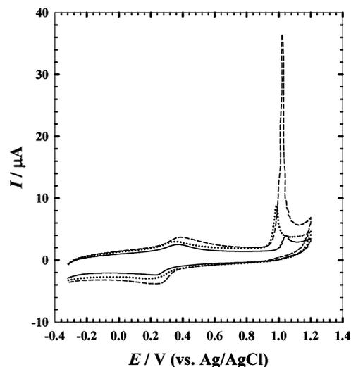
Fig. 1. CVs of 4.76 × 10<sup>-5</sup> mol L<sup>-1</sup> terazosin (in B–R buffer, pH 2) at GC electrode (—), in presence of 2.5 × 10<sup>-5</sup> mol L<sup>-1</sup> SDS without stirring (●●●), and after stirring for 5 min (---). Scan rate 100 mV s<sup>-1</sup>.
