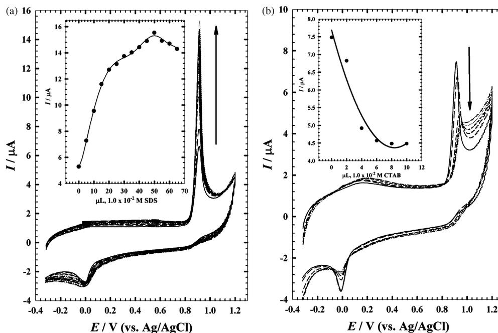
Fig. 3. (a) Effect of successive addition of SDS (increments add  $1.0 \times 10^{-5}$  mol L $^{-1}$  SDS of each addition) on the voltammetric response of terazosin in universal buffer, pH at GC electrode. Scan rate 100 mV s $^{-1}$ . (b) Effect of successive addition of CTAB (increments add  $4.0 \times 10^{-6}$  mol L $^{-1}$  CTAB of each addition) on the voltammetric response of terazosin in universal buffer, pH 5 at GC electrode. Scan rate 100 mV s $^{-1}$ .
