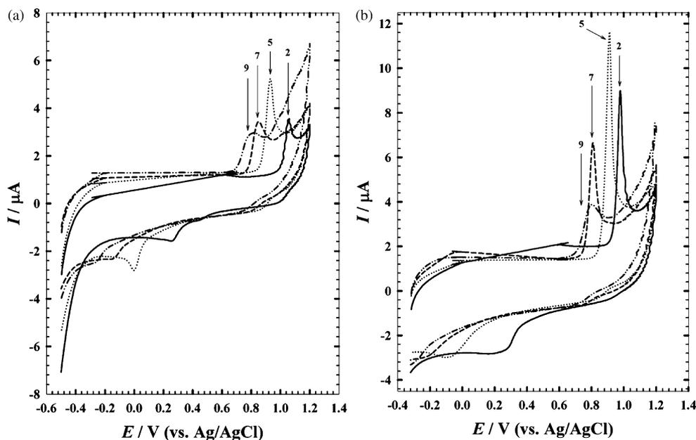
Fig. 2. (a) Effect of pH on the response of  $4.76 \times 10^{-5} \text{ mol L}^{-1}$  terazosin at GC electrode. pH 2(—), pH 5(●●●●), pH 7(---), pH 9(●-●-●-). Scan rate  $100 \text{ mV s}^{-1}$ . (b) Effect of pH on the response of  $4.76 \times 10^{-5} \text{ mol L}^{-1}$  terazosin at GC electrode in presence of  $2.5 \times 10^{-5} \text{ mol L}^{-1}$  SDS. Scan rate  $100 \text{ mV s}^{-1}$ . pH 2(—), pH 5(●●●●), pH 7(---), pH 9(●-●-●-).
