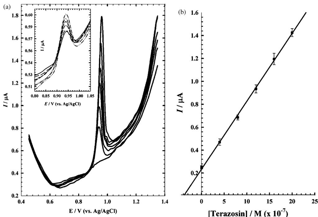
Fig. 6. (a) DPV of different concentrations of terazosin, insert ( $4.0 \times 10^{-8}$  mol L<sup>-1</sup> to  $2.4 \times 10^{-7}$  mol L<sup>-1</sup>), main ( $4.0 \times 10^{-7}$  mol L<sup>-1</sup> to  $2.4 \times 10^{-6}$  mol L<sup>-1</sup>) in presence of  $2.5 \times 10^{-5}$  mol L<sup>-1</sup> SDS, universal buffer (pH 2.0). (b) Standard addition plot of Itrin<sup>®</sup> in buffer pH = 2.
