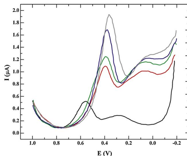
**Fig. 4.** SWVs of dopamine imprinted film after dipping in  $100 \mu\text{mol L}^{-1}$  of dopamine solutions at different values of pH: 1.0 (—), 3.0 (—), 5.0 (—), 7.0 (—), 9.0 (—).
