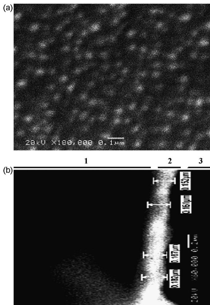
**Fig. 8.** Scanning electron microscope image of (A) sol-gel material used in the imprinting processes and (B) the side image of the sol-gel film coated on the surface of glassy carbon electrode. (1) Substrate edge, (2) sol-gel film and (3) air.
