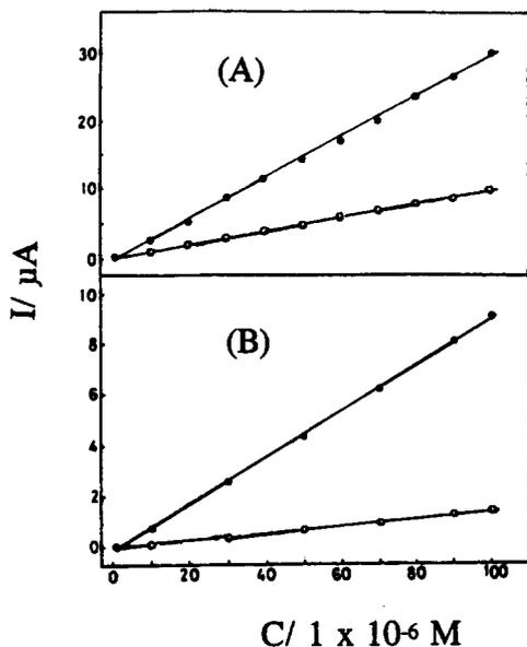
Fig. 6. Flow injection–amperometric detection calibration curves for (a) catechol and (b) ascorbic acid at P3MT (●) and Pt (○) electrodes. Sample size, 20  $\mu\text{l}$ ; mobile phase, Sørensen buffer (pH 6.9); flow rate, 1.0  $\text{ml min}^{-1}$ ; working electrode potential, 0.500 V.
