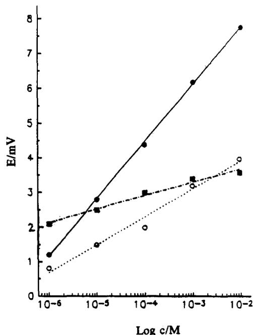
Fig. 24. BN-20-C-6 modified electrode under potentiometric FIA detection of various derivatives of catecholamines: ●, catechol; ○, L-dopa; ■, dopamine.
