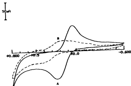
Fig. 12. Cyclic voltammograms of a 0.5 mM catechol + 0.1 M  $\text{Na}_2\text{HPO}_4$  (pH 7.5) solution at a P3MT electrode: curve A, untreated; curve B, cycled in a 0.1 M  $\text{NaMnO}_4$  buffer solution prior to use.
