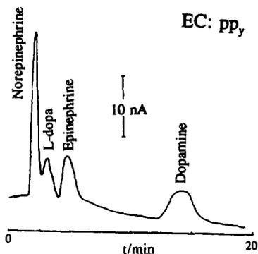
Fig. 9. Chromatogram of catecholamine mixture. Conditions as in Fig. 2 except poly-*N*-methylpyrrole used as working electrode; full scale is 50 nA.
