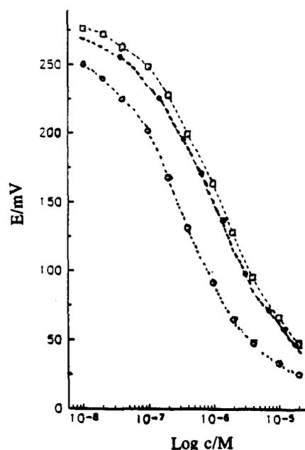
Fig. 23. BN-20-C-6 modified electrode under static potentiometric detection of various derivatives of catecholamines: □, L-dopa; ●, catechol; ○, dopamine.
