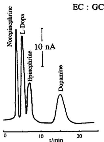
Fig. 8. Chromatogram of catecholamine mixture. Conditions as in Fig. 2 except glassy carbon used as working electrode; full scale is 50 nA.
