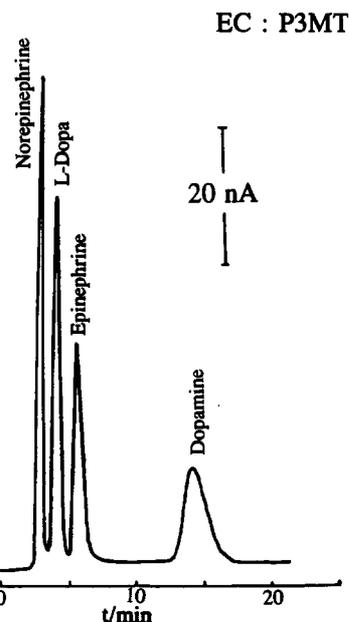
Fig. 7. Chromatogram of catecholamine mixture. Sample volume, 20  $\mu\text{l}$ ; PARTISIL 5 ODS-3 column; mobile phase, 0.15 M monochloroacetic acid, pH 3.00, 26°C; 100 nA full scale; flow rate, 1.5  $\text{ml min}^{-1}$ ; chart speed, 10  $\text{mm min}^{-1}$ ; detector BAS CV-1B; 0.55 V with P3MT working electrode.
