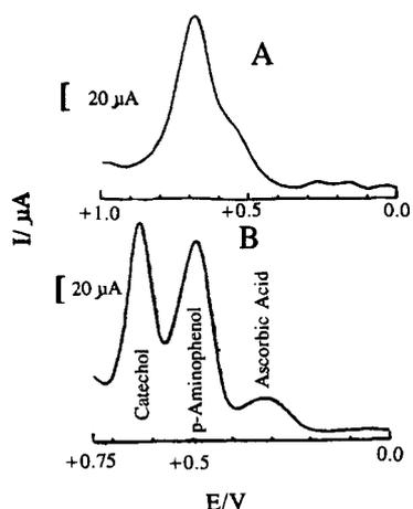
Fig. 2. Differential pulse voltammogram of a ternary mixture ( $5 \times 10^{-3}$  M of each) of ascorbic acid, *p*-aminophenol and catechol at (a) glassy carbon and (b) P3MT electrodes. Scan rate,  $4 \text{ mV s}^{-1}$ ; amplitude,  $25 \text{ mV}$ ; electrolyte, Sörenson buffer (pH 6.9).
