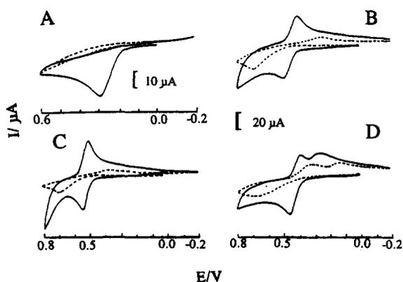
Fig. 1. Cyclic voltammograms for  $5 \times 10^{-3} \text{ M}$  (a) ascorbic acid, (b) dopamine, (c) catechol and (d) *p*-aminophenol at P3MT-coated (—) and bare platinum (----) electrodes. Scan rate,  $50 \text{ mV s}^{-1}$ ; electrolyte,  $0.1 \text{ M H}_2\text{SO}_4$ .
