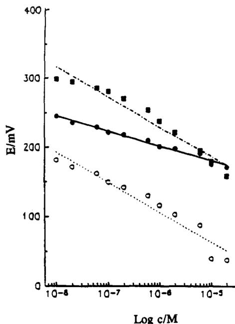
Fig. 22. DB-18-C-6 modified electrode under static potentiometric detection of various derivatives of catecholamines: ●, L-dopa; ○, catechol; ■, dopamine.
