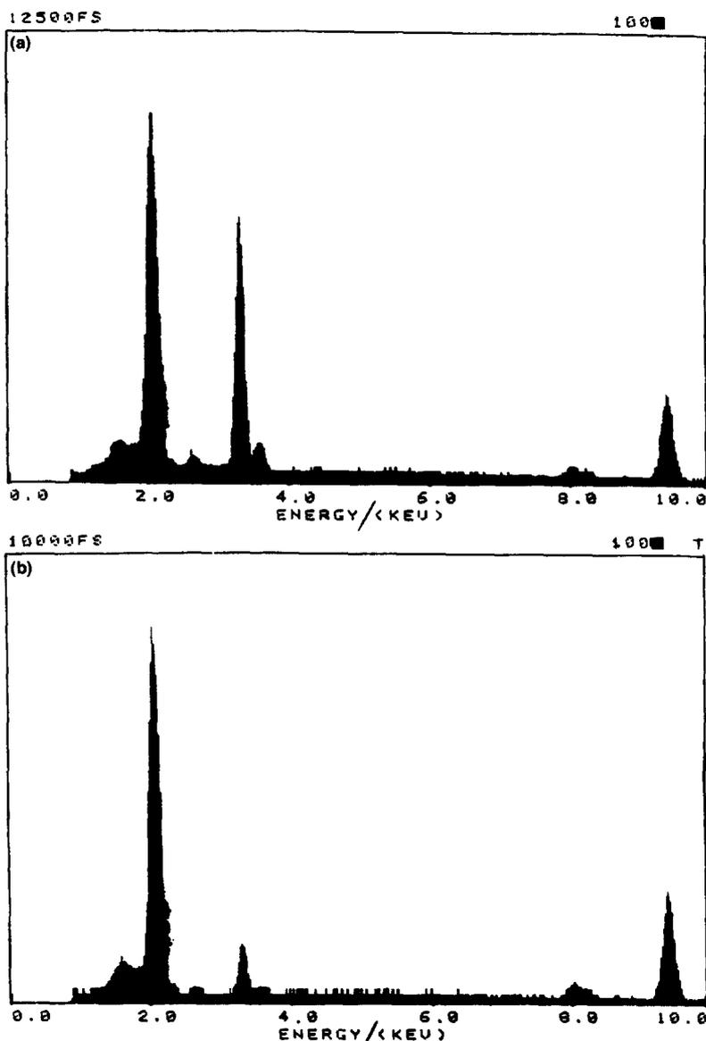
Fig. 27. EDAX analysis before and after electrode response to catecholamines: (a) 0.1 M phosphate buffer (pH 9.4); (b) buffer +  $10^{-6}$  M dopamine or  $10^{-6}$  M epinephrine.
