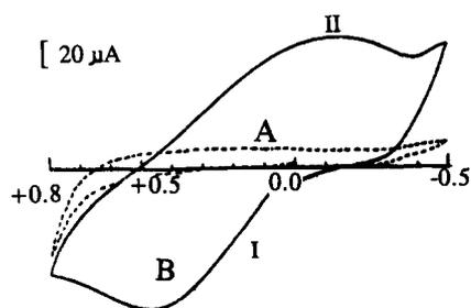
Fig. 3. Cyclic voltammetric response of P3MT grown on Pt in the absence (curve A) and in the presence (curve B) of  $1 \text{ mM NADH}$  (in  $0.01 \text{ M H}_2\text{SO}_4$ ). Scan rate,  $50 \text{ mV s}^{-1}$ . I, anodic; II, cathodic.
