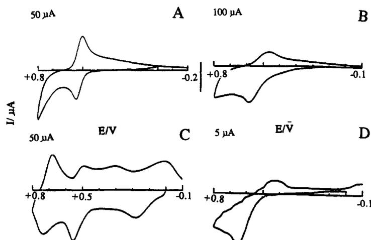
Fig. 11. Cyclic voltammety of 5 mM catechol in 0.1 M  $\text{H}_2\text{SO}_4$  at (a) P3MT, (b) poly-*N*-methylpyrrole, (c) polyaniline, PAn, and (d) polyfuran, PF electrodes. Scan rate, 50  $\text{mV s}^{-1}$ . All films were prepared under similar conditions.
