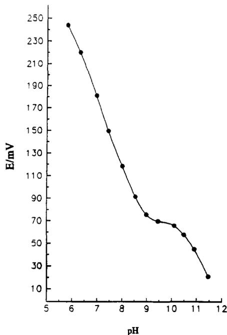
Fig. 15. The pH dependence of potentiometric response of poly-(binaphthyl-20-crown-6) electrodes. 0.1 M K phosphate buffer;  $10^{-6}$  M dopamine and/or epinephrine.
