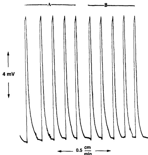
Fig. 26. Examples of FIA signals obtained on the modified DB-18-C-6 electrode. Sample size, 20  $\mu$ l; mobile phase, potassium phosphate buffer (pH 9.4); curves A,  $10^{-2}$  M catechol; curves B,  $10^{-2}$  M catechol +  $10^{-2}$  M ascorbic acid.
