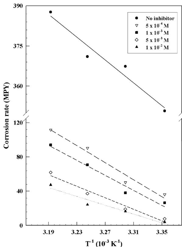
Fig. 4. Relation between the rate of corrosion of stainless steel of type 316 in  $H_2SO_4$  vs.  $1/T$ ; MPY (milli-inch per year)  $\approx 0.00219 \text{ mA cm}^{-2}$ .
