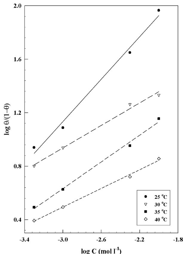
Fig. 2. Adsorption isotherm of TCH for the different concentrations of inhibitor studied at different temperatures.
