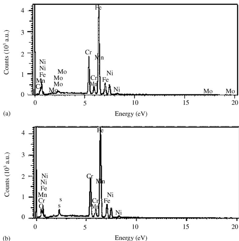
Fig. 8. Energy-dispersive X-ray analysis of the steel samples exposed to 0.5 M  $\text{H}_2\text{SO}_4$  (a) and 0.5 M  $\text{H}_2\text{SO}_4 + 1.0 \times 10^{-3}$  M TCH (b).
