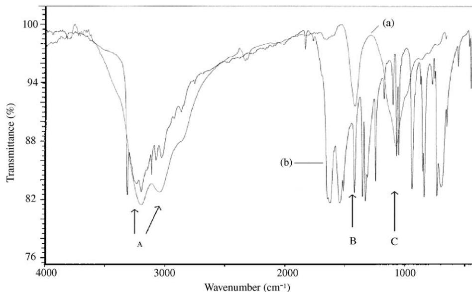
Fig. 9. FT-IR obtained by reflectance from the surface of the steel (a) and from a conventional transmission experiment (b) of TCH.
