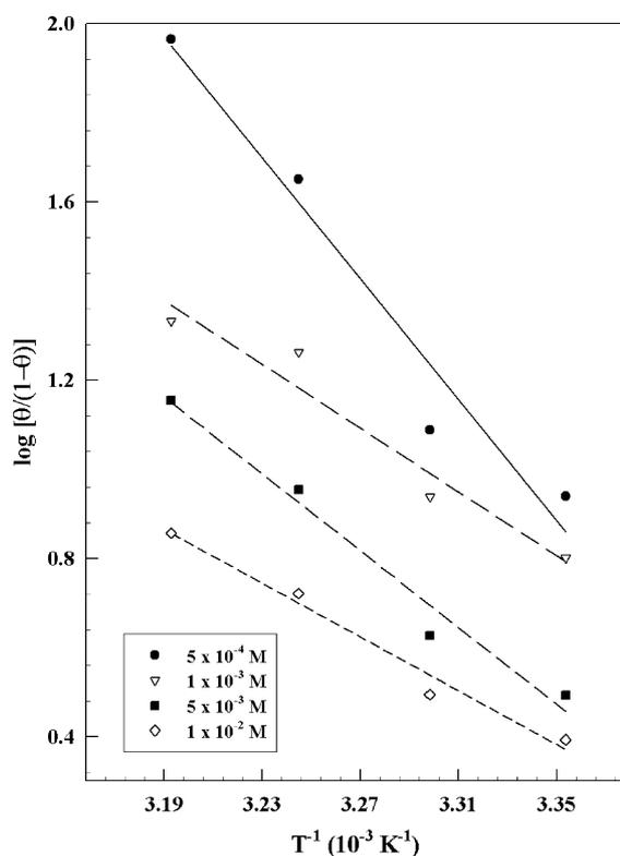
Fig. 3. Plot of  $\log[\theta/(1-\theta)]$  vs.  $1/T$  for given concentration values of TCH at stainless steel of type 316.
