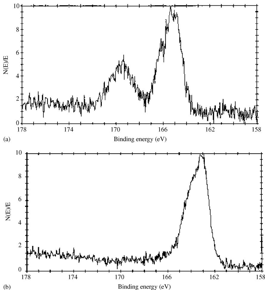
Fig. 10. XPS data of stainless steel samples exposed to the inhibitor (a) and a platinum substrate exposed to the same inhibitor (b).
