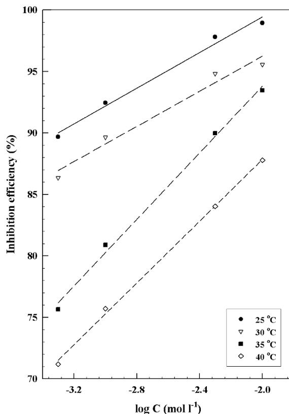
Fig. 1. Inhibition efficiency for different concentration of TCH at different temperatures.
