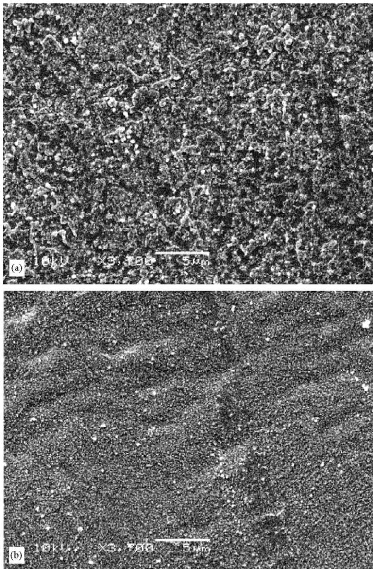
Fig. 6. SEM images showing surface features of stainless steel 316 exposed to 0.5 M  $\text{H}_2\text{SO}_4$  in absence (a) and presence (b) of  $1.0 \times 10^{-3}$  M TCH for 10 min under potential step polarization conditions.
