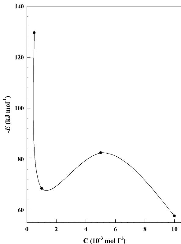
Fig. 5. Activation energy vs. inhibitor concentration.
