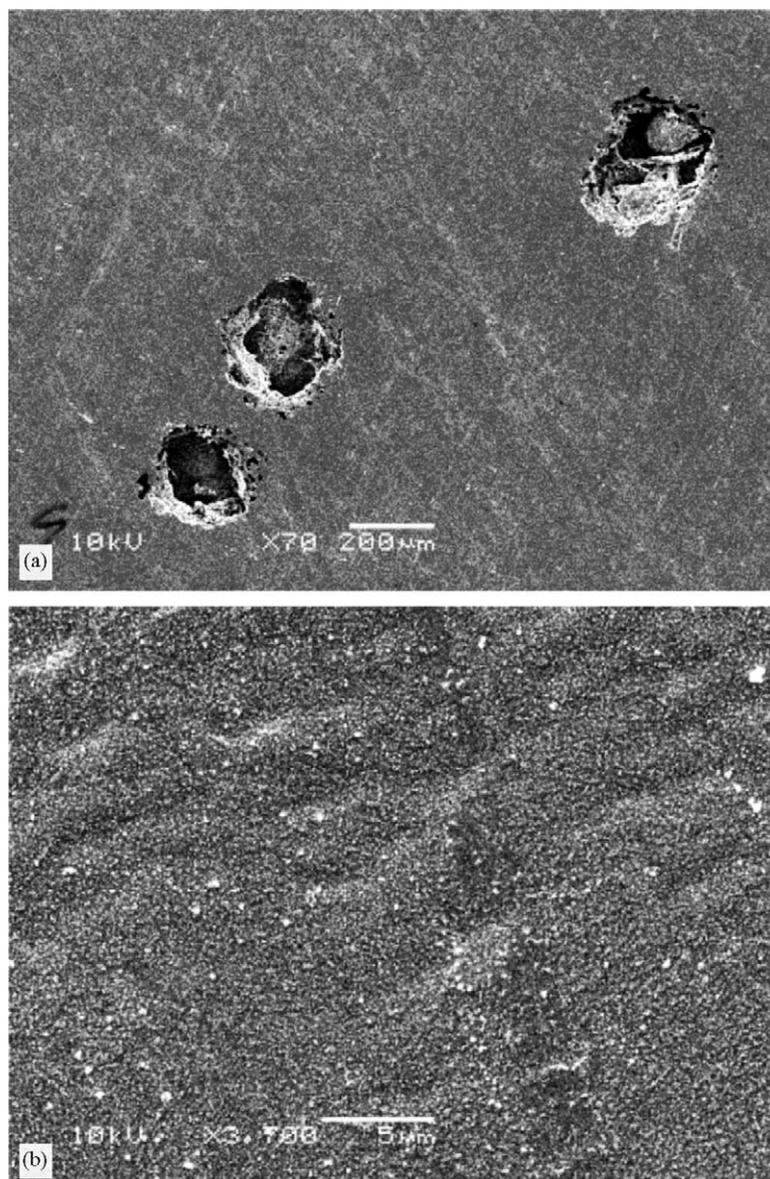
Fig. 7. SEM images of the specimen surface after exposure to a 0.01 M NaCl-containing 0.5 M H<sub>2</sub>SO<sub>4</sub> in absence (a) and presence (b) of inhibitor.
