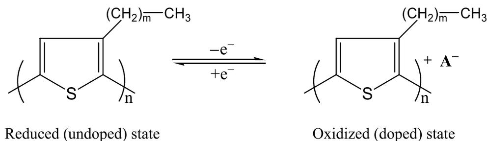
**Fig. 1.** Oxidation/reduction of poly(3-alkylthiophenes).  $m = 7, 11, 15$  (octyl-, dodecyl-, hexadecyl-)  $\text{A}^-$ : counter anion
