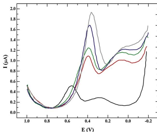
**Fig. 4.** SWVs of dopamine imprinted film after dipping in  $100 \mu\text{mol L}^{-1}$  of dopamine solutions at different values of pH: 1.0 (—), 3.0 (—), 5.0 (—), 7.0 (—), 9.0 (—).
