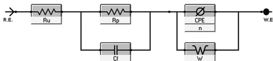
**Fig. 7.** Electrochemical equivalent circuit for EIS measurements.
