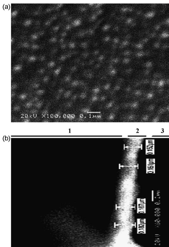
**Fig. 8.** Scanning electron microscope image of (A) sol-gel material used in the imprinting processes and (B) the side image of the sol-gel film coated on the surface of glassy carbon electrode. (1) Substrate edge, (2) sol-gel film and (3) air.
