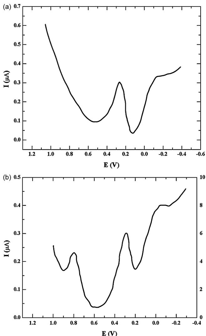
**Fig. 3.** SWV signal characteristic for dopamine imprinted film after dipping in (A) binary mixture of dopamine and tyrosine and (B) binary mixture of dopamine and tyramine. Rebinding binary solutions are  $50 \mu\text{mol L}^{-1}$  with respect to template molecules.
