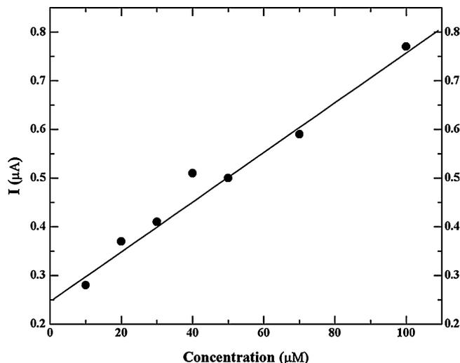
**Fig. 5.** Current response (SWV) of dopamine imprinted film as a function of the concentration of dopamine in the rebinding solution.
