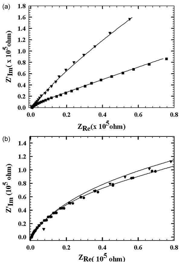
**Fig. 6.** (A) Nyquist plots of dopamine imprinted films tested in dopamine solution compared to the signal after testing in PBS. (B) Nyquist plots of dopamine imprinted films tested in tyrosine solution compared to the signal after testing in PBS.
