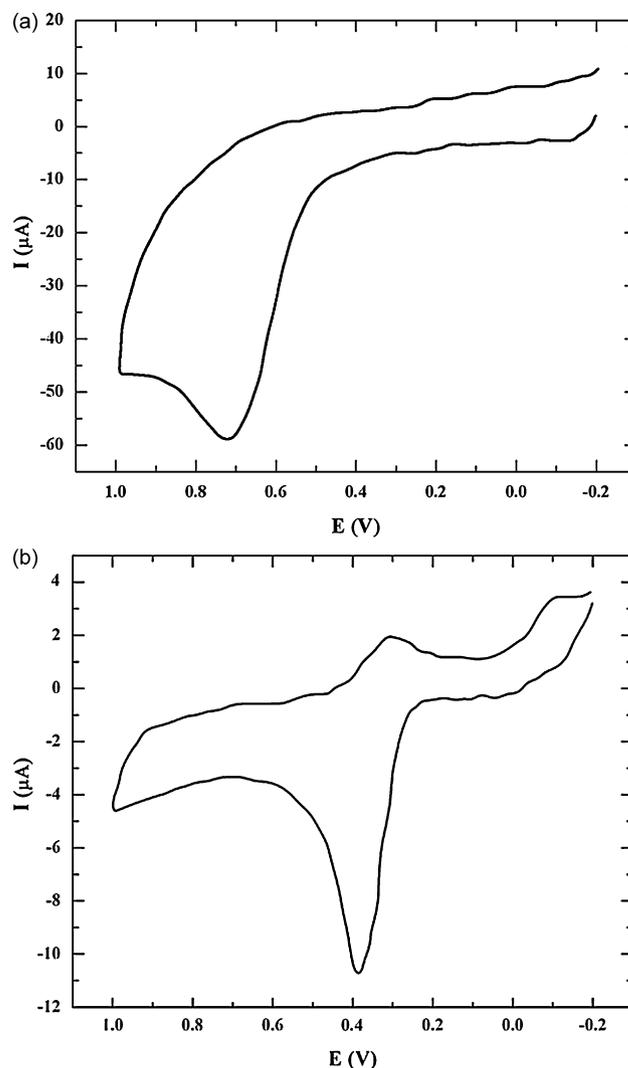
Fig. 1. Cyclic voltammograms of tyramine (A) and dopamine (B) molecularly imprinted sol–gel films spin coated on the surface of glassy carbon electrodes cycled in PBS ( $\text{pH } 7.2$  and  $10 \text{ mmol L}^{-1}$ ) versus  $\text{Ag/AgCl}$  reference electrode.
