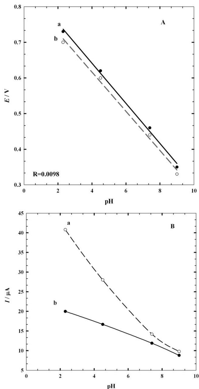
Fig. 2. A) A plot of the anodic peak potential values as a function of pH value of the solution at PEDOT/Pt electrode (a) in presence and (b) in absence of SDS. B) A plot of the anodic peak current values as a function of pH value of the solution at PEDOT/Pt electrode (a) in presence and (b) in absence of SDS.
