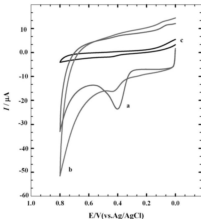
Fig. 1. Cyclic voltammograms of  $5.0 \times 10^{-4} \text{ mol L}^{-1}$  morphine/ $0.1 \text{ mol L}^{-1}$  BR, pH 7.4, at (a) PEDOT/Pt electrode in the presence of SDS, (b) PEDOT/Pt electrode (c) Pt electrode, at scan rates  $50 \text{ mV s}^{-1}$ .
