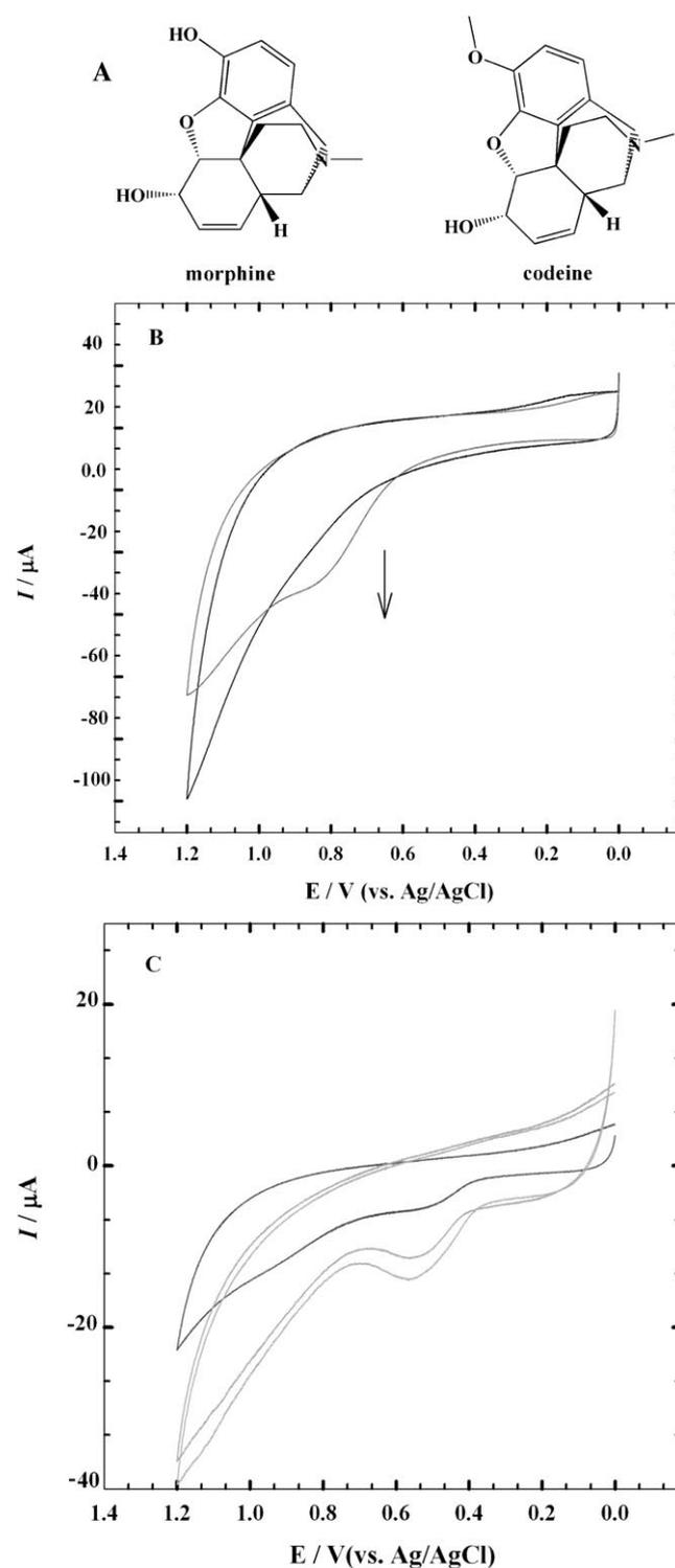
Fig. 6. A) Molecular structure of morphine and codeine. B) Cyclic voltammograms for 5 mmolL<sup>-1</sup> codeine in 0.1 molL<sup>-1</sup> BR pH 7.4 at PEDOT/Pt electrode (a) in 0.1 molL<sup>-1</sup> 100 μL SDS (b). C) Cyclic voltammograms for equimolar solution 0.5 mmolL<sup>-1</sup> for each of MO and codeine in 0.1 molL<sup>-1</sup> BR pH 7.4, at PEDOT/Pt electrode at pH 7.4 with two successive additions of 100 μL 0.1 molL<sup>-1</sup> SDS, scan rate 50 mV s<sup>-1</sup>.
