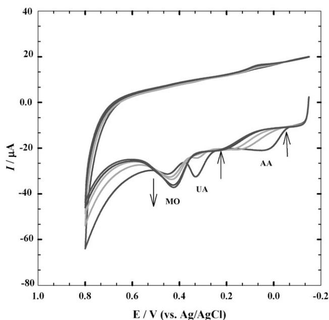
Fig. 5. Cyclic voltammograms for  $50 \text{ mmol L}^{-1}$  ascorbic acid,  $5 \text{ mmol L}^{-1}$  uric acid and  $0.5 \text{ mmol L}^{-1}$  MO in  $0.1 \text{ mol L}^{-1}$  BR pH 7.4 at PEDOT/Pt electrode with successive additions of  $0.1 \text{ mol L}^{-1}$  SDS (0–100  $\mu\text{L}$ ).
