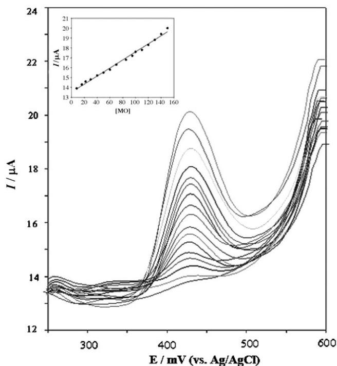
Fig. 7. SWV for the successive additions of 10  $\mu\text{L}$  of 2  $\text{mmolL}^{-1}$  morphine tablets solution to the buffer pH 7.4 containing 100  $\mu\text{L}$  SDS. Calibration curve of MO for concentrations from (8  $\mu\text{molL}^{-1}$ –150  $\mu\text{molL}^{-1}$ ) (Inset).
