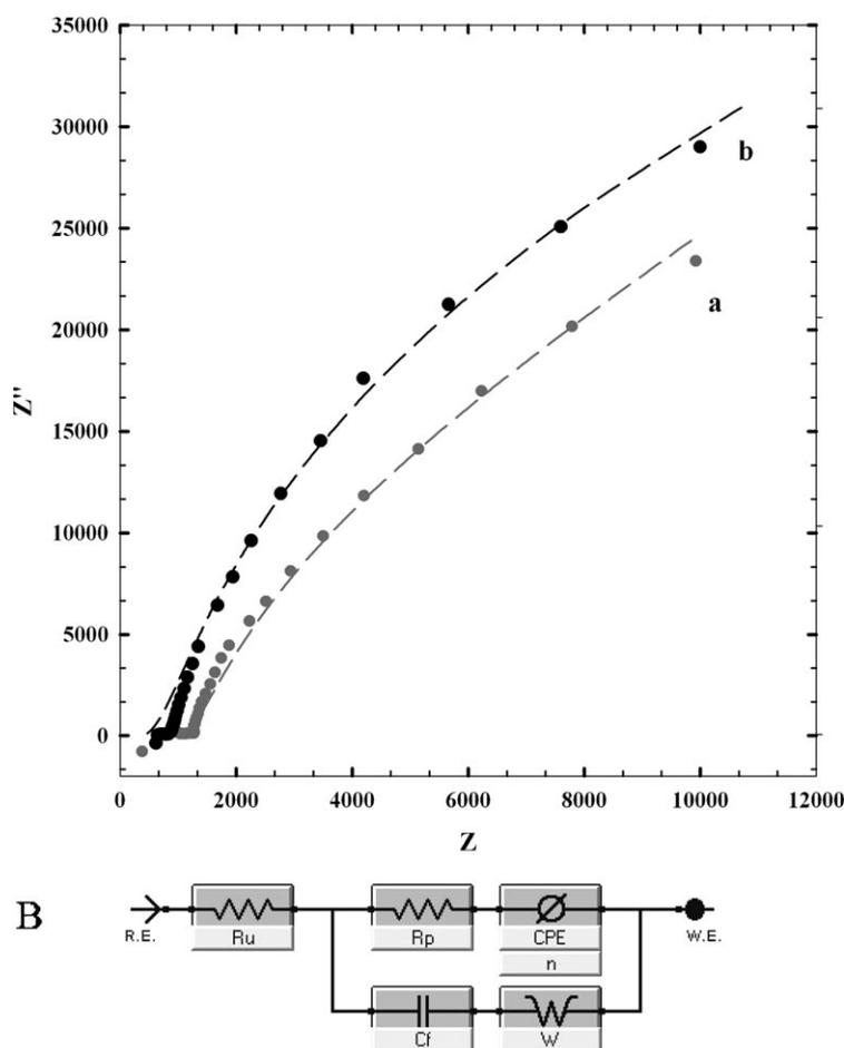
Fig. 8. A. Nyquist diagrams ( $-Z''$  vs.  $Z'$ ) for the EIS measurements at PEDOT/Pt at potential 420 mV for 5 mmolL<sup>-1</sup> MO in 0.1 molL<sup>-1</sup> BR pH 7.4, (a) in presence of SDS and (b) in absence of SDS. Amplitude: 5 mV, frequency range: 0.1–100 000 Hz. B. The equivalent circuit.
