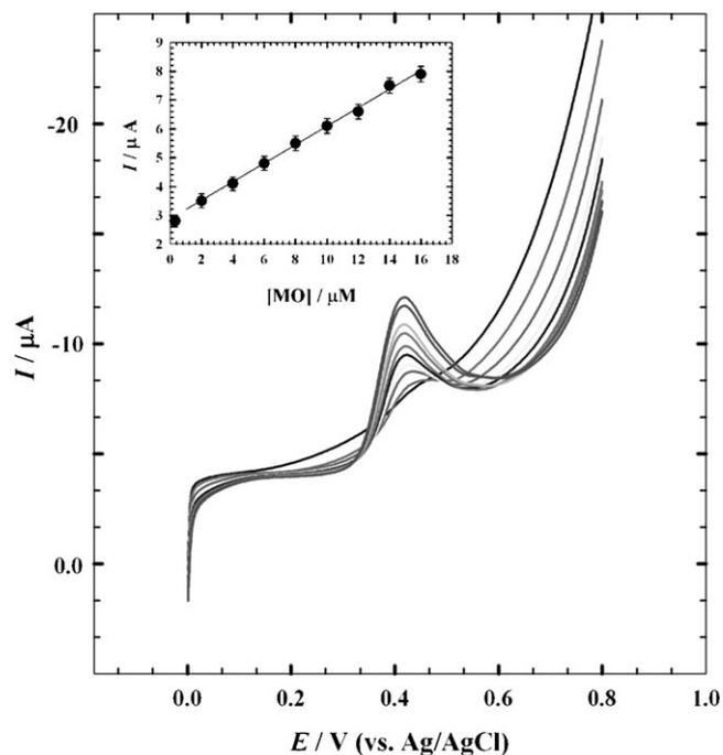
Fig. 3. LSVs for MO of different concentrations ( $0.3 \mu\text{molL}^{-1}$  to  $16 \mu\text{molL}^{-1}$ ) in  $0.1 \text{ molL}^{-1}$  BR pH 7.4 at PEDOT/Pt electrode in  $0.1 \text{ molL}^{-1}$   $100 \mu\text{L}$  SDS. Calibration curve of MO of concentrations from ( $0.3 \mu\text{molL}^{-1}$  to  $16 \mu\text{molL}^{-1}$ ) (Inset).
